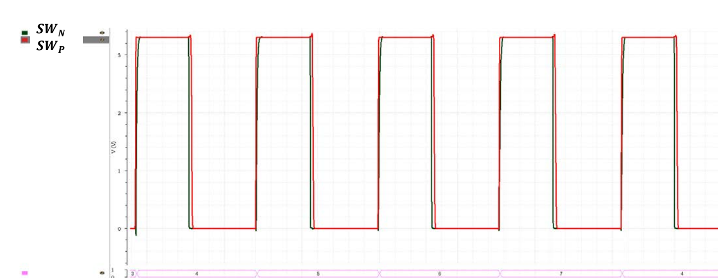
Fig 8. Power transistor switching voltage and dead time.
